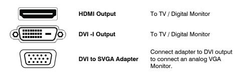
Attach the monitor or monitors to the rear of the recorder using the cable supplied by the monitor manufacturer. Refer to the monitor manual for detailed information on how to setup and use it.
